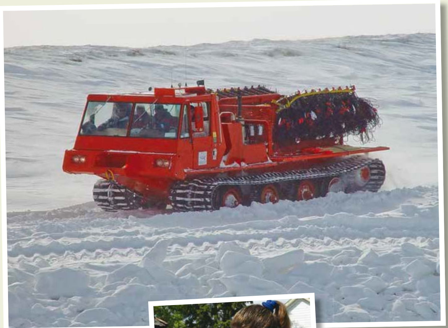
A line vehicle conducts seismic operations in the Mackenzie Delta, Northwest Territories.
