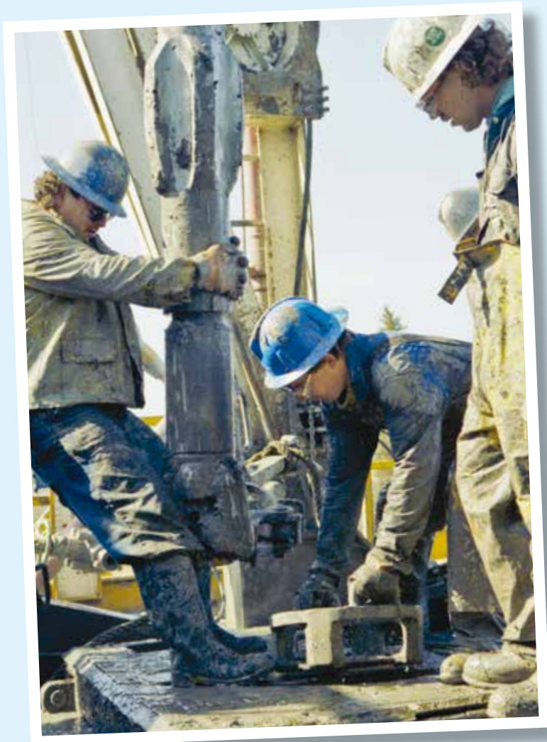
Roughnecks replace a drill bit.
