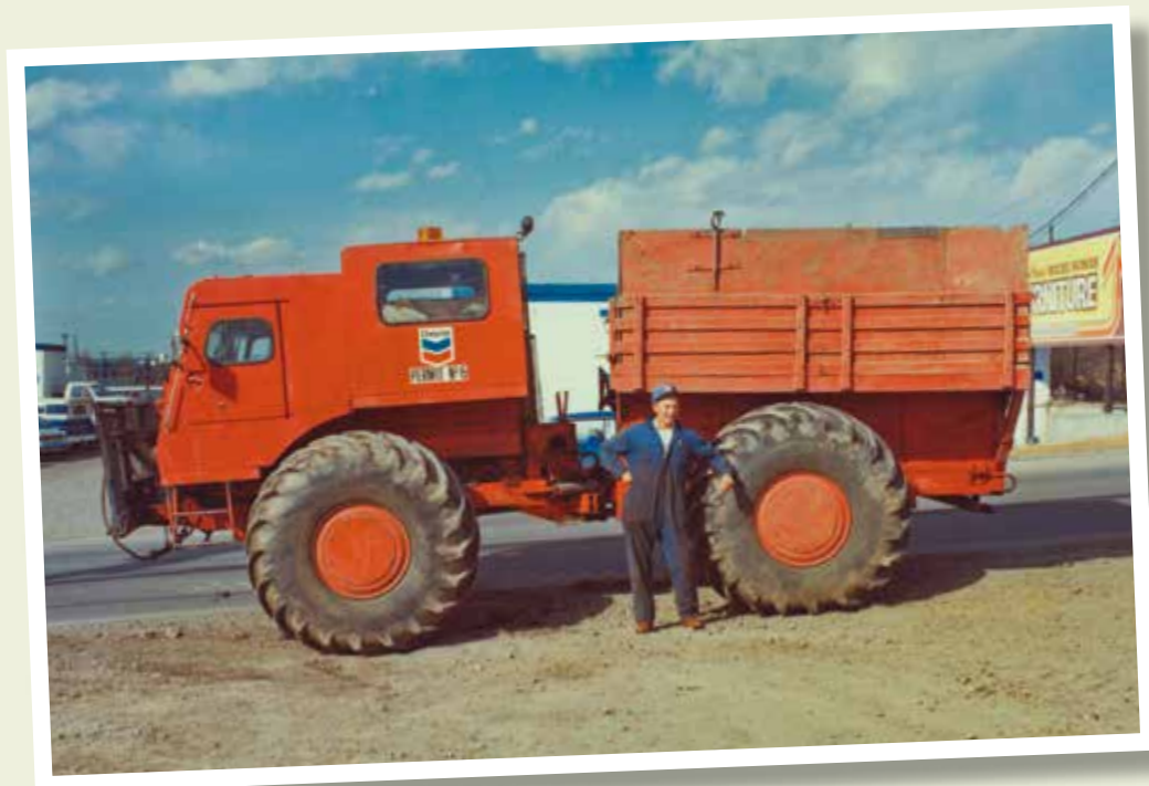
A seismic line buggy at the Chevron maintenance shop in Calgary in 1981.
